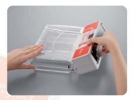
Power supply can be easily detached from gel electrophoresis tank by lifting it up.
